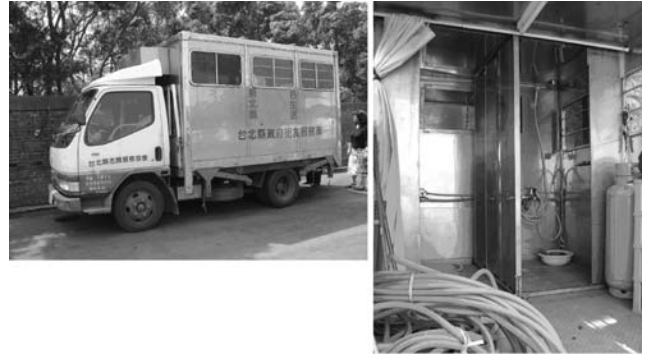
Photo 44. Exterior and interior of shower van (equipped with two showers and a hot water heater)
