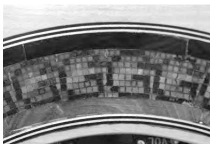
Fig. 2. Rosette of the Storyteller Guitar showing the dark rings of 45 million year old Metasequoia on the outside of the rosette, and light coloured rings of recently harvested Metasequoia from a tree growing in Guelph, Ontario, Canada.
