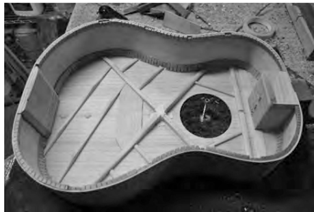
Fig. 8. Scalloped bracing of the top plate for Metasquoia # 2.
