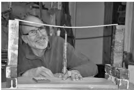
Fig. 5. Illustration of simple setup for measuring strength of wood samples.
