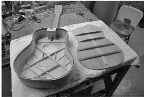
Fig. 7. Bracing pattern of the top plate for Metasequoia #1.
